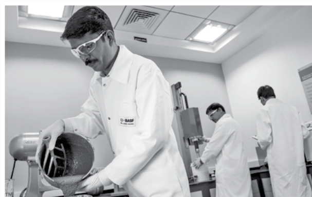
An R&D employee tests concrete additives which are used to change certain physical characteristics of concrete such as flowability. This helps enhance the concrete's performance under various conditions.
